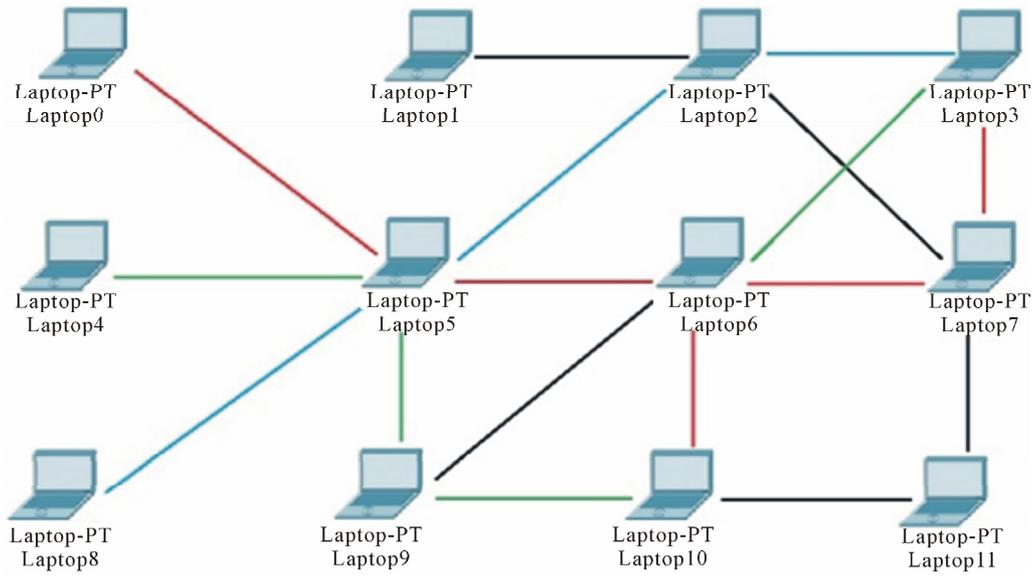
**Figure 2. Simulation topology with certain bandwidth, delay and Jitter for each link.**
